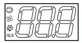
Red light = cold mode engaged (compressor working)
