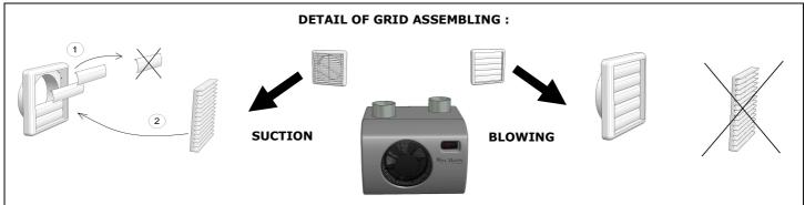
**ATTENTION!** Each module consists of two grids (blowing and suction). Care must be taken to adapt the type of grid.
